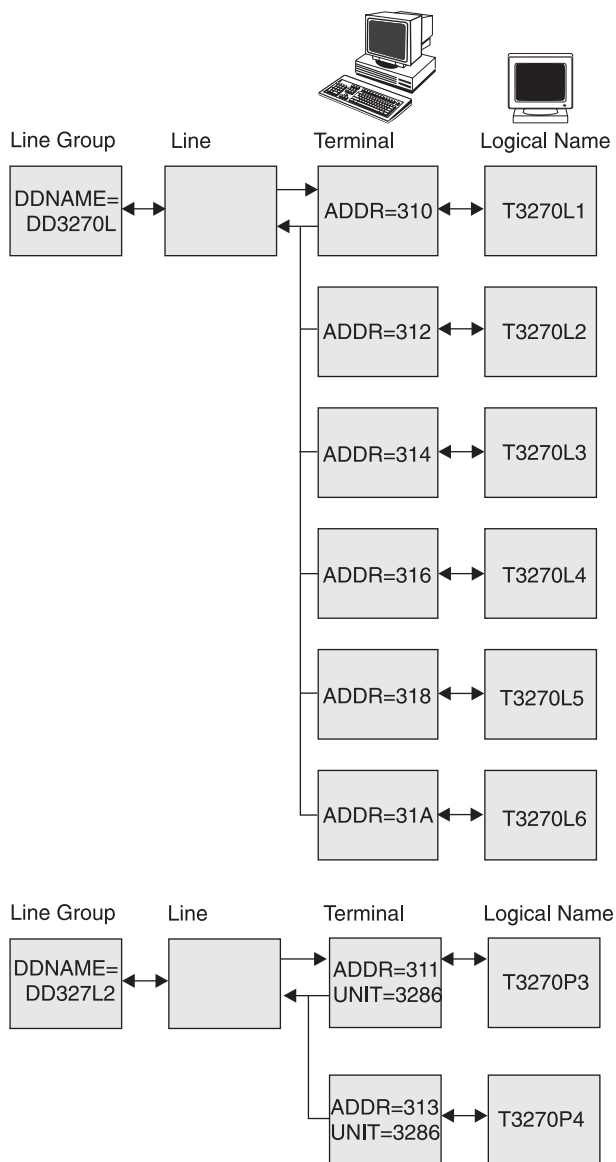
Figure 2. Configuration for 3270 Local Line Group
