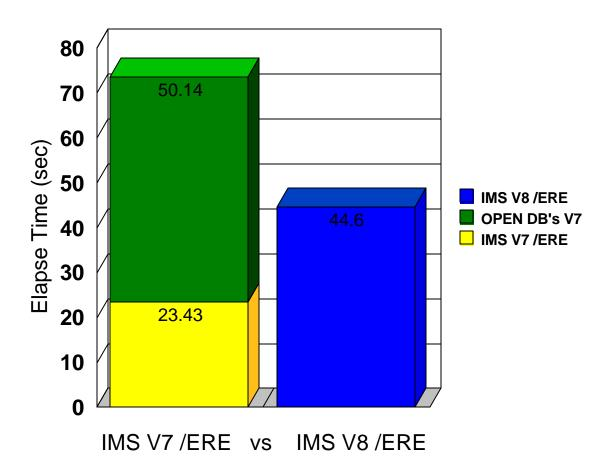
Figure 5.3 shows the improved database open time for IMS Version 8 when compared to IMS Version 7.
