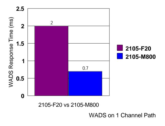
Figure 11.4: MSC via VTAM CTC - WADS I/O response time comparison
