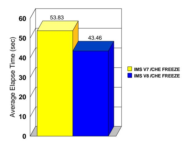
Figure 5.5 shows the improved shutdown time for IMS Version 8 when compared to IMS Version 7 when using the checkpoint dumpq command to stop IMS.
