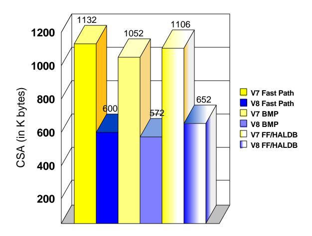
Figure 4.2 shows the reduction in CSA usage below the 16 MB line by IMS Version 8 relative to IMS Version 7 in an APPC environment. The statistics show IMS Version 8 uses less CSA than IMS Version 7 in both Full Function and Fast Path environments when driven through APPC.
