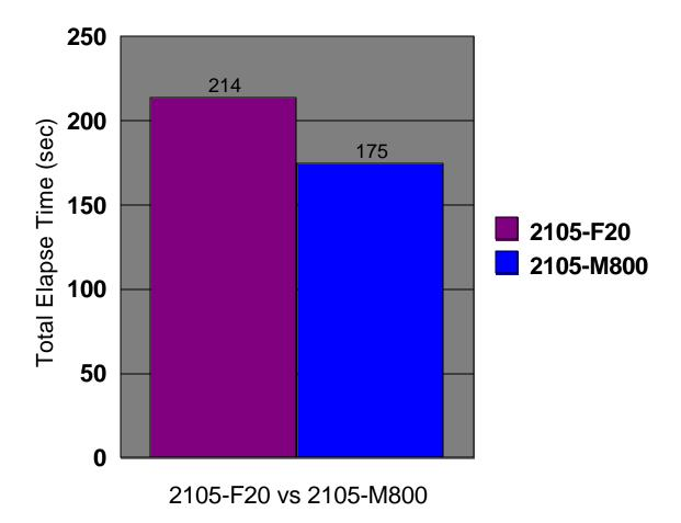
Figure 11.6 shows the reduced batch window requirement for database reorganization when the target database resides on ESS M800 when compared to the target database residing on ESS F20.
