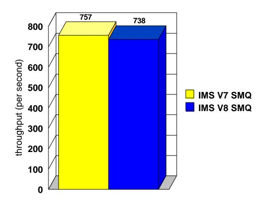
Figure 3.3 shows the IMS transaction rates achieved when the CPU utilization was at a steady state of 70% busy while running the DCW workload. The statistics show the transaction rates achieved in IMS Version 8 relative to IMS Version 7. The statistics show IMS Version 8 Fast Path transaction processing capacity is nearly equivalent to IMS Version 7 with a variance of only 2.2%.
