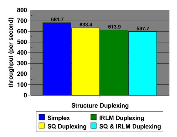
Figure 8.2 shows the transaction rates achieved when IMS Version 8 was active with data sharing and Shared Message Queues. The statistics show the impact to IMS transaction rates when enabling structure duplexing of the shared message queues structure and the IRLM global lock structure on a remote coupling facility. The statistics show that overhead for duplexing multiple structures is less than the aggregate overhead incurred for duplexing the individual structures.
