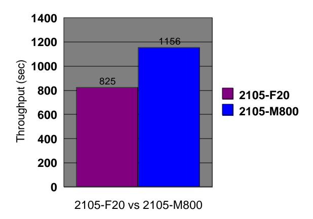
Figure 11.4 shows the improved WADS I/O response time achieved when the WADS resides on the ESS M800 when compared the WADS residing on the ESS F20. This constitutes the first time IMS WADS I/O is measured in sub-millisecond times.
