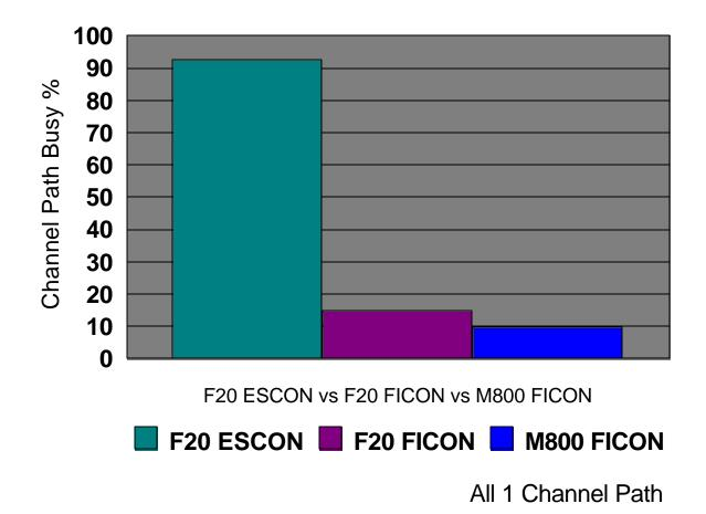
Figure 11.2: OLDS logging - Channel utilization comparison
