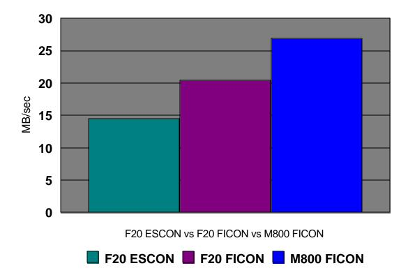
Figure 11.2 shows the improvement in channel utilization by ESS 800 compared to ESS F20 with both ESCON and FICON channels. The statistics show the ESS M800 reduces the channel utilization when compared to ESS F20.
