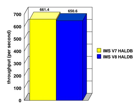
Figure 3.2 shows the IMS transaction rates achieved when the CPU utilization was at a steady state while running the DSFF workload using shared queues. The statistics show the transaction rates achieved in IMS Version 8 relative to IMS Version 7. The statistics show IMS Version 8 Full Function transaction processing capacity is nearly equivalent to IMS Version 7 with a variance of 2.5%.
