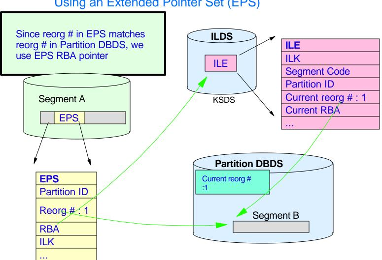
Using an Extended Pointer Set (EPS)
