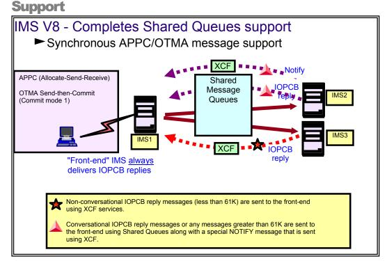
With IMS V8, the restriction on synchronous messages has been removed. The new capability allows any IMS in a Shared Queues group to process <u>synchronous</u> APPC and OTMA inbound messages, enabling the APPC/OTMA workload to be distributed amongst the Shared Queue group. In prior releases, synchronous messages had to be processed on the IMS system that maintained the connection to the client ("front-end").
