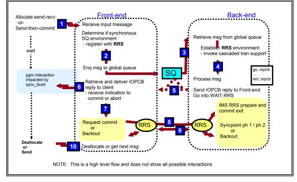
This visual provides a general flow of a synchronous message as it is processed in an IMS Shared Queues environment:
