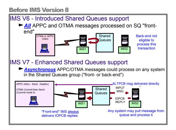
When Shared Queues support was introduced in IMS V6, the processing of <u>all</u> APPC and OTMA messages (synchronous and asynchronous) was restricted to the front-end IMS. As shown in the picture, a "front-end" is the IMS to which the APPC or OTMA client is connected and a "back-end" is any other IMS in the Shared Queues group.
