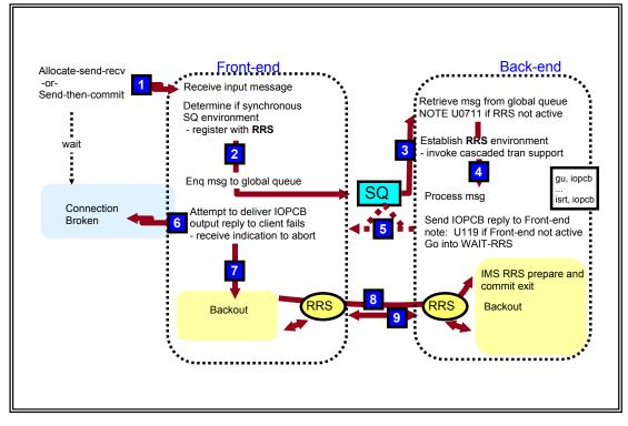
This visual provides a general flow of a synchronous message as it is processed in an IMS Shared Queues environment and the response cannot be returned by the front-end:
