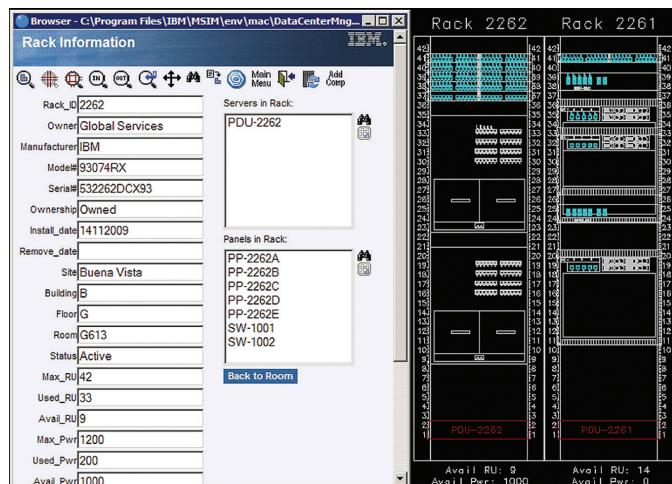
A rack elevation view enables managers to drill into the rack contents and view the associated attributes, including point-to-point connectivity.
