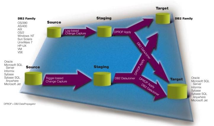
The IBM replication solution enables full-refresh and change propagation across a heterogeneous database environment.
