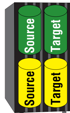
Figure 2- 11: Source and target pairs on alternate ranks
