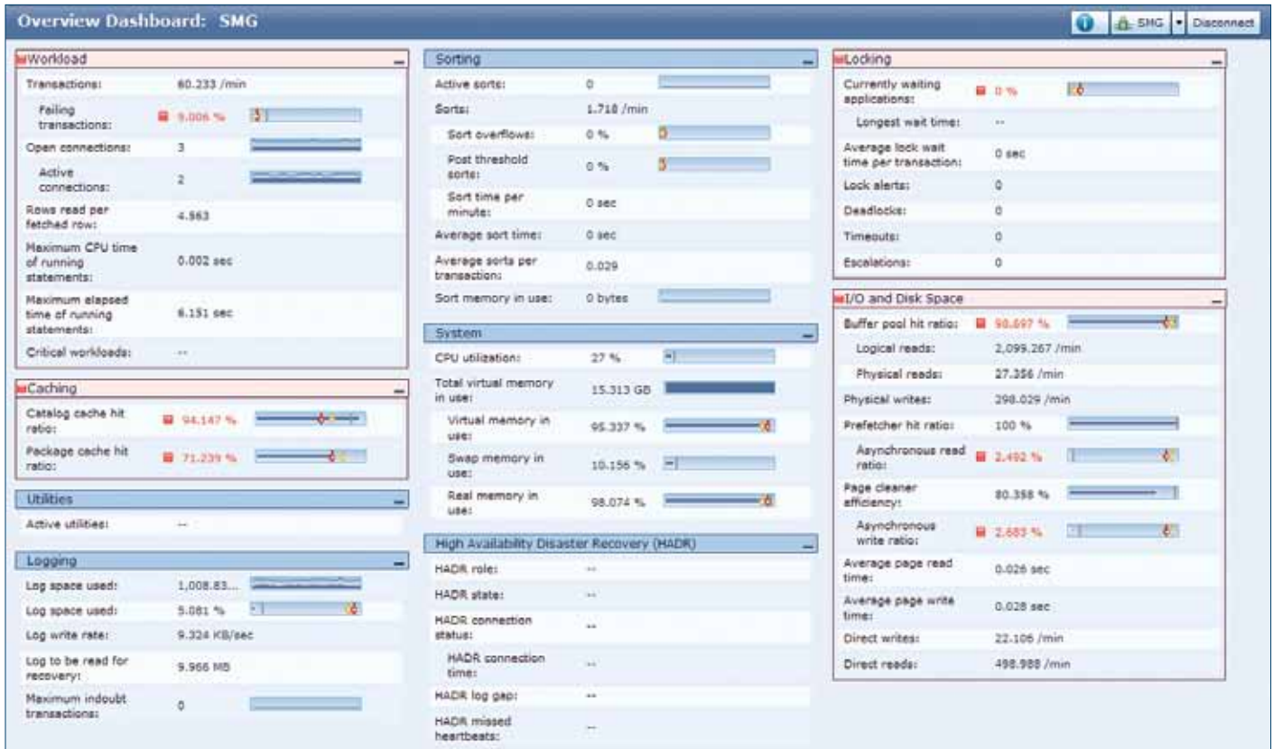
Figure 1: The InfoSphere Optim Performance Manager dashboard has a color-coded, web-based interface designed to quickly alert users to problematic areas. Once a problem has been identified, specific diagnostics and details are provided to focus on that area. Integration with InfoSphere Optim products provides the resolution needed to correct the problem.
