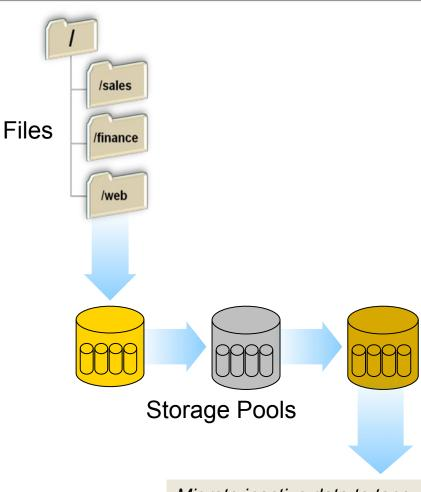
Migrate inactive data to tape, tape lib, or de-duplication device via TSM Server
