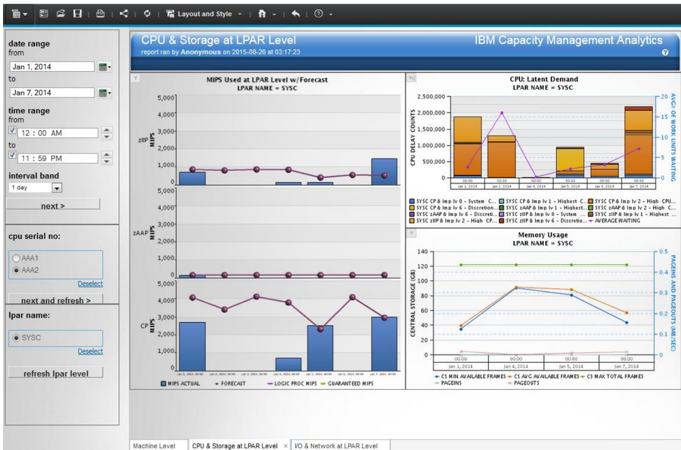
Figure 60: zServer Monitoring Dashboard CPU & Storage at LPAR Level tab example
