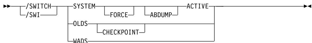
*/SWITCH for an alternate XRF subsystem*
