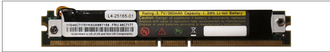
Figure 3-27 The battery backup unit for the ServeRAID-MR10ie (CIOv) Controller
