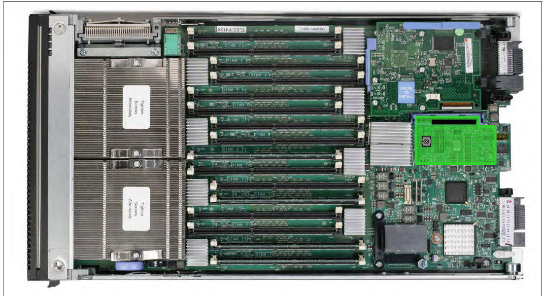
Figure 3-74 The HX5 type 7873 showing the CIOv I/O Expansion card position
