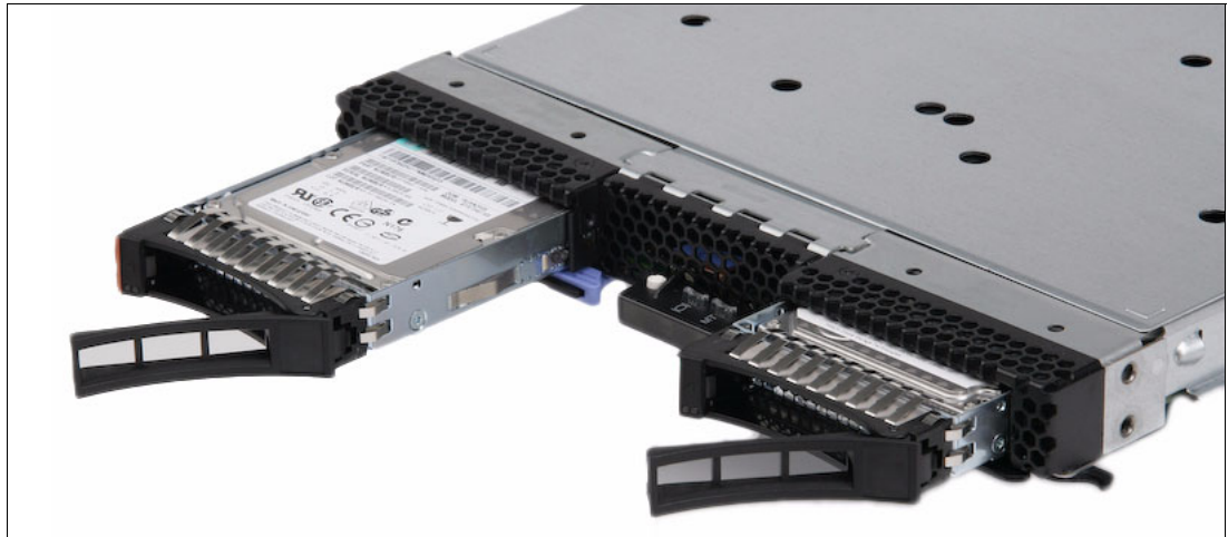
Figure 3-40 The HS22 showing the front hot-swap disk drive bays
