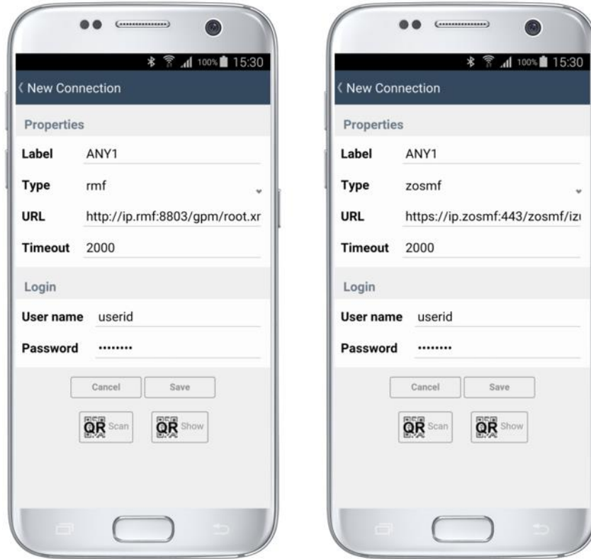
Figure 4: Definition of a New Connection
