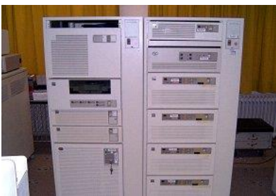
A rack mounted, air-cooled ES/9221 with rack mounted disk and tape.
