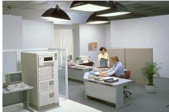
An IBM 9370 system in an office environment with rack mounted CPU and disks.
