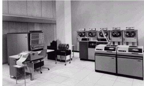
A typical IBM System/360 Model 30 with CPU and console, reel-to-reel tape drives, card reader/punch, and disk drives
