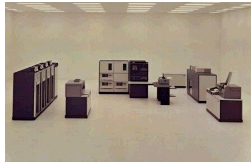
A typical IBM System/370 Model 135 system with reel-to-reel tape, card punch, CPU and disk drives, TP controller, printer, and card reader. Addition of a TP controller to the picture shows that by the early 1970s, communications was becoming an important part of S/370 systems.
