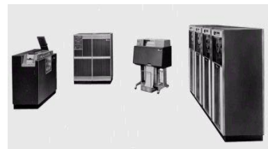
A typical IBM 1401 System with card reader/punch, CPU, printer, and reel-to-reel tape drives.
