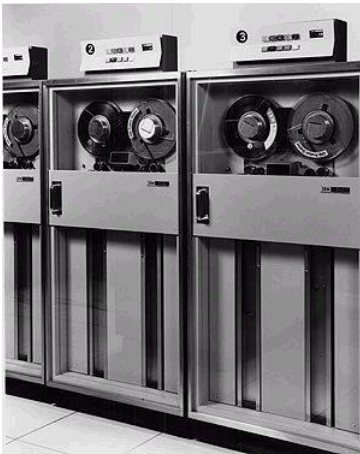
Reel-to-reel tape drives - spinning tapes were the public 'image' of DP in the early days of computing.
