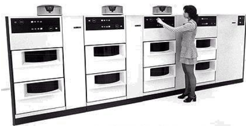
A full eight drive IBM 3330 unit. Each disk contained 100 MB per removable pack. Operators were frequently called upon to mount and unmount packs.
