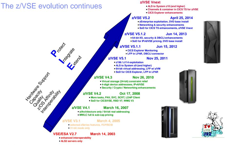
z/VSE V3 is 31-bit mode only. It does not implement z/Architecture, and specifically does not implement 64-bit mode capabilities. z/VSE is designed to exploit select features of IBM System z10, System z9, and zSeries hardware.
