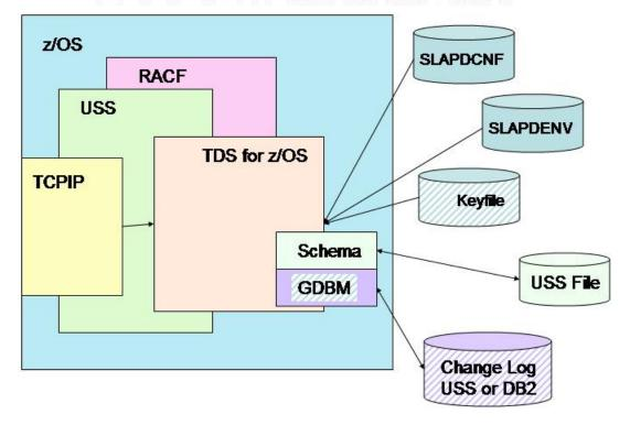
The z/OS TDS server is built with information in the configuration file (SLAPDCNF), the environment variables file (SLAPDENV), and the schema definitions. The keyfile will hold any digital certificates and public/private keys for the z/OS TDS server. And the GDBM is the change log for the z/OS TDS server.
