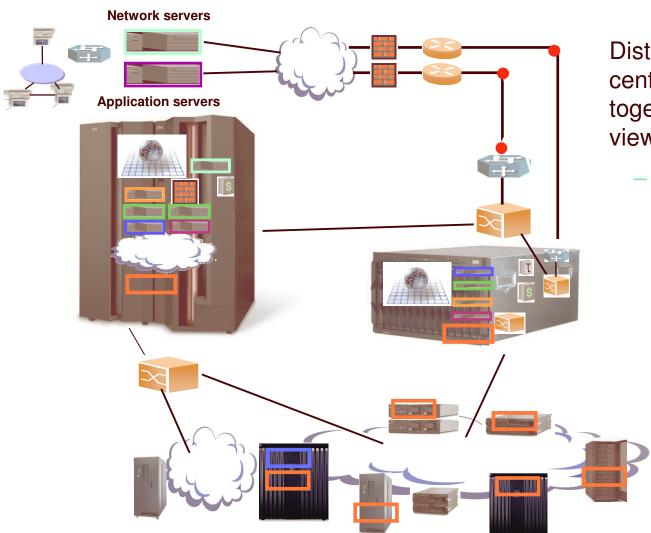
Distributed servers and centralized servers can work together with a centralized view of data
