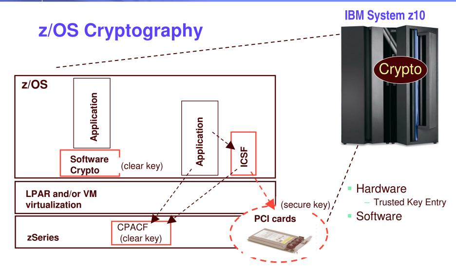
Crypto accessible via multiple language paths; from assembler for clear key crypto to CCA, OCSF, and Java™ interfaces to secure key HW assisted crypto.
