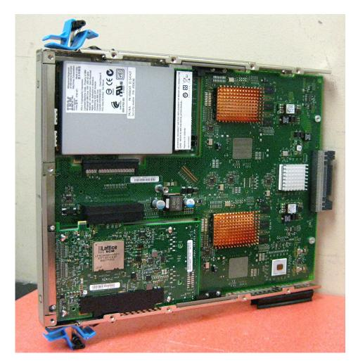
If card is tampered with (especially silver case, upper left of photo) then the keys are inaccessible.
