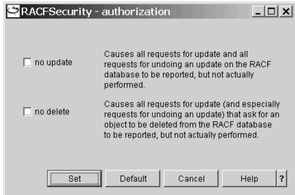
Figure 9. RACFSecurity authorization policy panel
