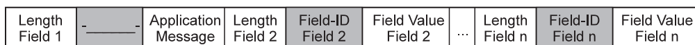
Figure 7. MQIA Message Consisting of More Than One Data Field and One Application Message
