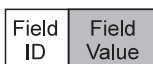
Figure 5. MQIA Message Consisting of One Data Field Preceded by a Field Identifier
