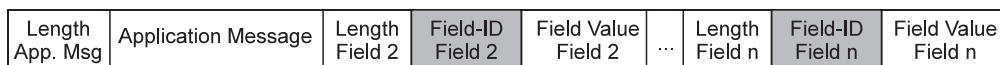
Figure 6. MQIA Message Consisting of One Application Message and at least One MERVA-related Data Field
