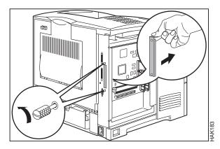
4. Remove the cover from the NIC interface connector, if present. Insert the card into the connector, lining up the faceplate with the slot.
