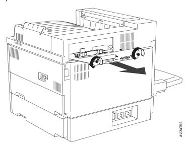
4. Loosen and remove the screws that hold the slot cover. Remove the cover and store it for future use.
