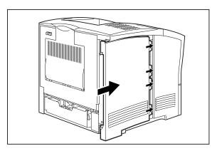
c. Tighten the screws at the top and the bottom of the cover.
