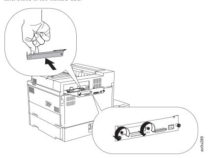
5. Insert the card into its socket, lining up the faceplate with the slot.
