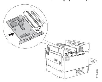
6. Tighten the thumbscrews on the network card.
