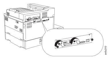
7. Slide the controller card back into the printer. Tighten the thumbscrews at the left and right ends of the controller card.
