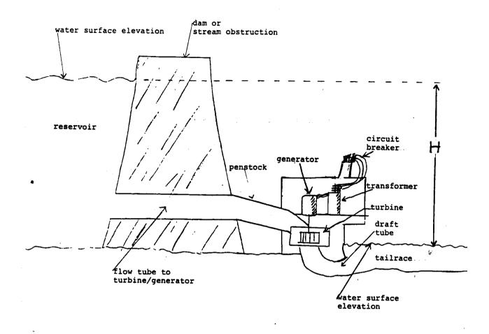
Figure 1. Typical Micro-Hydroelectric System Showing Major Components and Hydraulic Head
