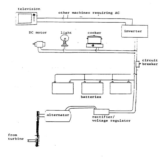
Figure 3. A Low-Voltage DC Electric Power System
