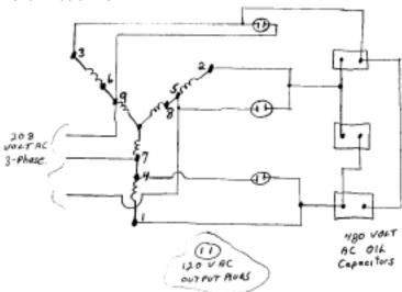
The correct size capacitor can be selected from the following graph. Each plug will be capable of about 1/3 of the generators rating. There will be approximately 480 volts ac at the capacitors, so use care not to touch them when the generator is operating CHART #2
