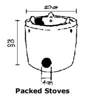
Natural Draft Stove The husks are fed into the stove above the fire and fall down a slanted grate as they burn. The air intake is located under this grate, forcing all air drawn into the stove to pass through the burning fuel. The stove ash is raked out from below the grate. The Thailand and Philippine models below are widely used in the provinces of Bulacan, Laguna and Cavite. The Philippine model comes in different sizes and is widely available in local markets.
