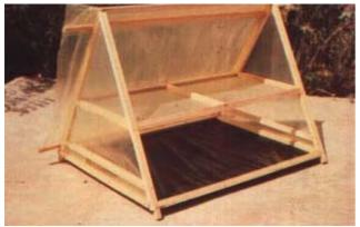
84. Inside the dryers, the tomato slices will be placed on trays made of slatted plastic and mosquito netting.
