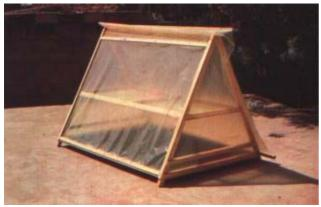
83. This one is simpler, cheaper to build and mobile. But the drying system is the same. First of all, the plastic retains the heat of the sun and, secondly, the air circulates inside, coming in at the bottom and going out at the top.
