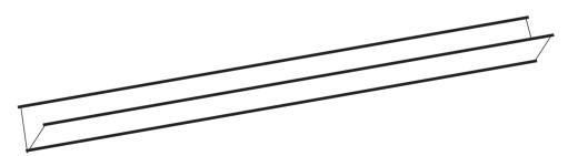
□ If you use a piece of wood, hollow it out along its length, or attach two planks of wood together lengthways in a "V" shape. Water will flow along this groove. Apply tar or wax to the joint so that water will not be lost through the joint.
