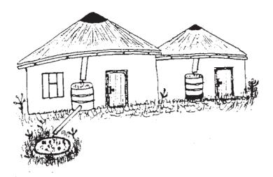
You may install a pipe to channel the water from the lowest point on the gutter into a storage container.
