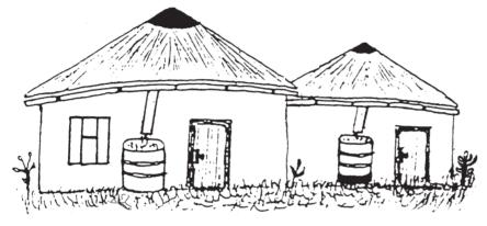
It does not matter what the roof is made of. Water collected from thatched roofs is often discoloured and is usually contaminated, so it should not be used for drinking. Use this water only for watering plants. Tile or metal roofs give the cleanest water.
