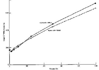
Sulfurized jojoba oil in general lubricants. Laboratory tests have demonstrated that jojoba can match the exceptional lubricating qualities of sperm oil. (Source: H. Gisser)
