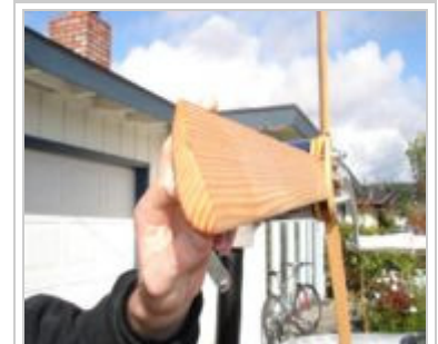
Finished blade shape
