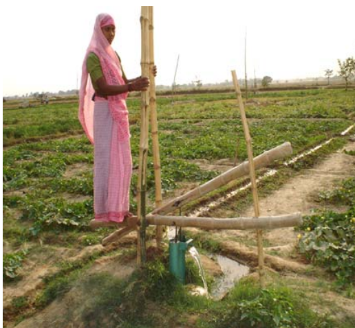
Figure 4: Using the bamboo treadle pump in Kapilvastu, Nepal. Photo: Practical Action Nepal.
