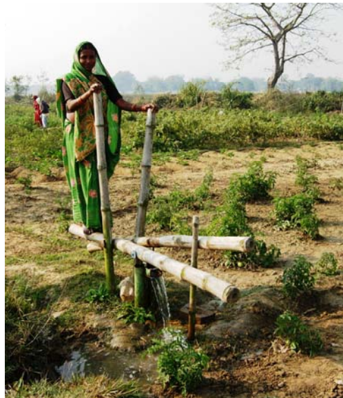
Figure 1: Bamboo treadle pumps are used for irrigation in Nepal. Photo: Practical Action / Sandra Gibson.
