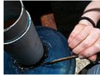
Fig. 3d: Bri sealing water bottle with caulk
