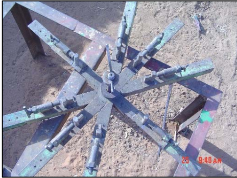
Picture 4: A completed wheel jig
