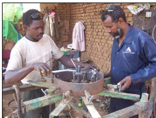
Picture 8: The wheel rim is placed in the jig and measured for accuracy
