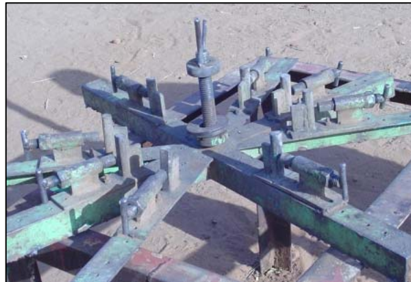
Picture 5: A completed wheel jig from above (Note: The diagonal parts of the jig base should be at 45 degree angles as shown in the technical drawings).
