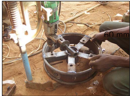
Picture 10: A makeshift pillar drill used for drilling the holes in the spokes
