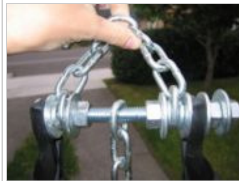
Figure 2: Bolt to attach the trailer to the rear bike rack
