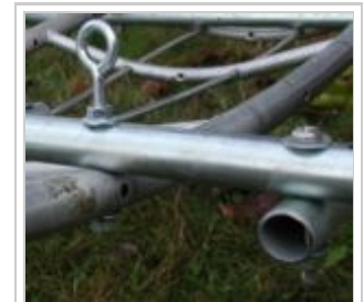
Left: eye-bolt. Right: standard bolt
