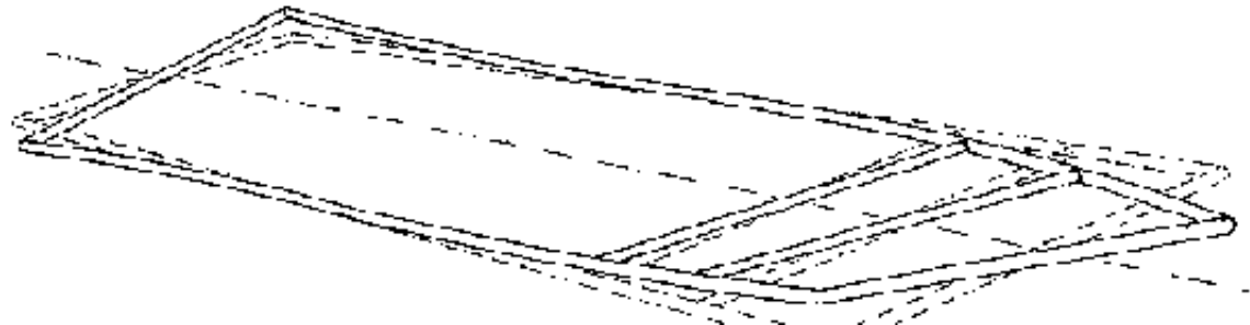
Fig. 25: Action of the torsional moment on the frame
