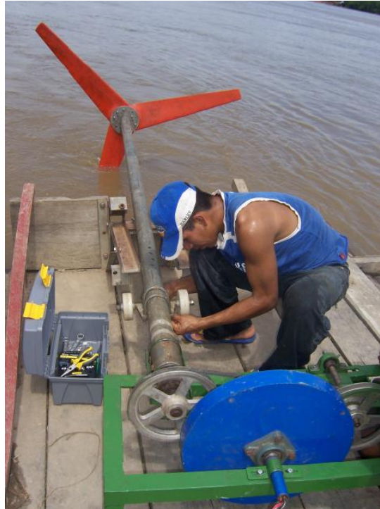
Figure 3: A robust and simple design was developed for remote locations. A simple permanent magnet generator was designed (painted blue). Photo: Soluciones Prácticas.
