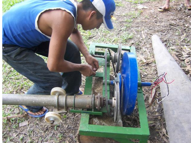
Figure 4: Setting up the fan belt and permanent magnet generator . Photo: Soluciones Prácticas.
