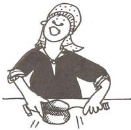
Fig. 4.3 Cutting a block of clay into half and slamming the top half onto the bottom half (wedging)
