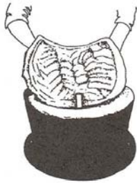
Fig. 4.5 Putting the slabs in the mould and pushing the slabs against the inside walls
