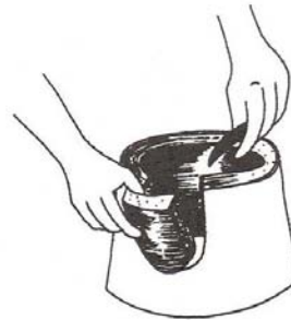
Fig. 4.18 Removing the clay
