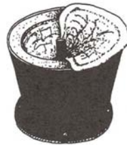
Fig. 4.5 Putting the slabs in the mould and pushing the slabs against the inside walls
