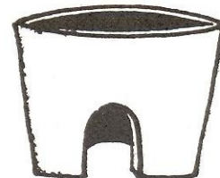
Fig. 4.19 The stove liner
