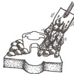
Fig. 7.5 Putting stones and soil around the liner
