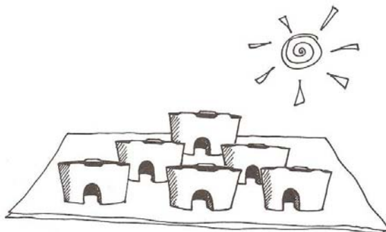
Fig. 4.26 Drying the liners
