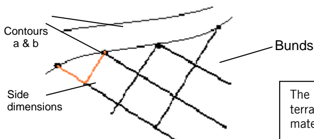
Figure 6: Laying out the bunds using contours
