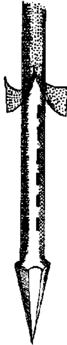
FIG. 14-3. BRASS-JACKED DRIVE POINT
