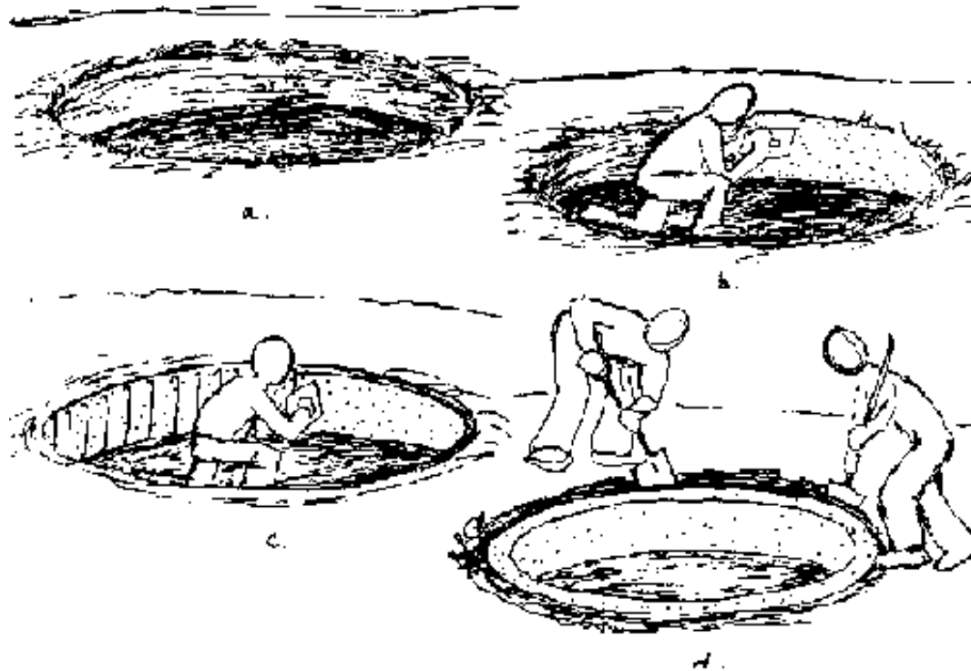
FIG. 8-12. CASTING CONCRETE RINGS IN EARTH FORMS
