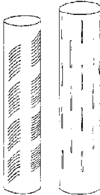
FIG. 15-2. LOCALLY MADE SLOTTED PLASTIC PIPE
