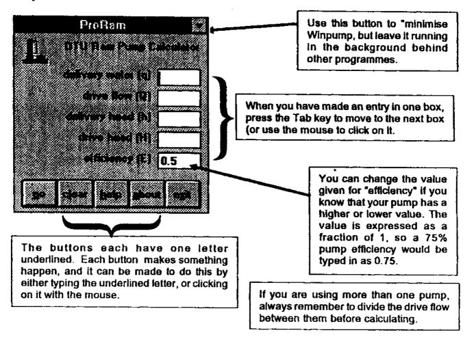
When you have made one calculation and wish to make another, click on the "clear" button. All the values will disappear, except for 0.5, which is the default pump efficiency.
