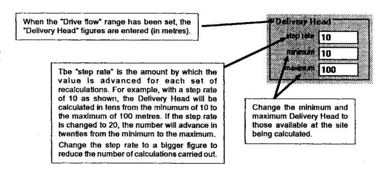
After setting the Step rates and the maximum and minimum entries for Drive Head (H), Drive Flow (Q) and Delivery Head (h) at a site, click on the "go" button to start making calculations.
