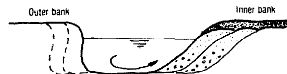
Fig. 26. Erosion and sedimentation in the bends of a meandering river.
