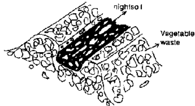
Fig. A1.2. Placing nightsoil in a compost windrow (b)
