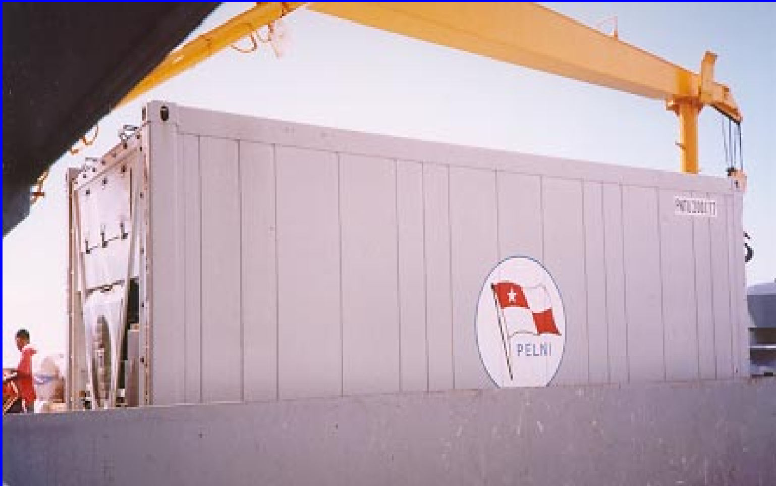
20-foot refrigerator container on the Dobonsolo.
