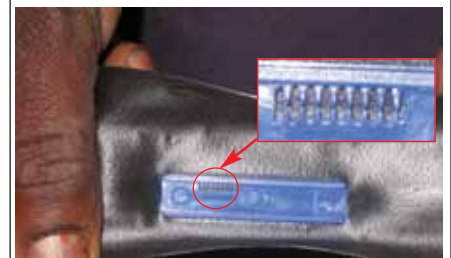
Inside a drip pipe: Only clean water can run out of the small holes shown (arrow)
