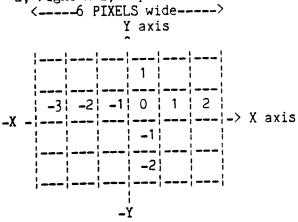
You can see that the center PIXEL in this 6X4 box is located in the lower left hand corner of the upper right hand quadrant.
