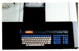
The *inbuilt printer* produces forms which are 8.5 inches (22.6 cm) wide—easy to work with and precisely the convenient size for most filing systems. Its 90 characters-per-second matrix printer is bi-directional for fast throughput.
