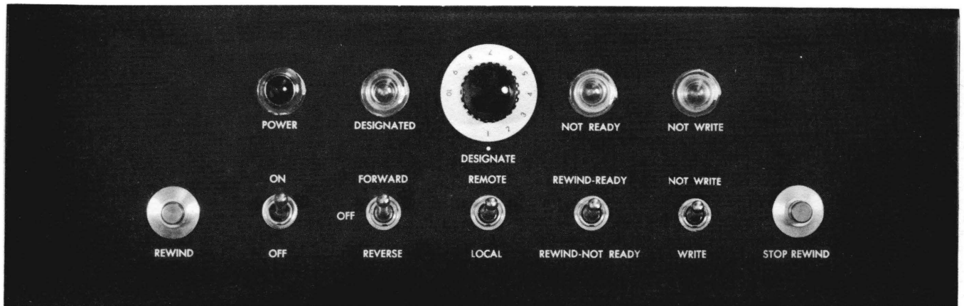
Figure 9-4. Tape Storage Unit Control Panel.
