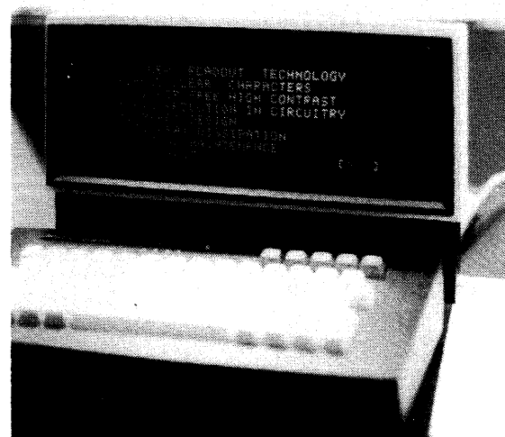
One or two Burroughs TD 700 Series display/keyboard units like this one can be used with an L 8000 or L 9000 for data entry into a dedicated magnetic tape cassette station, concurrently with program execution on the computer. This photograph was taken at a trade show, under very poor lighting conditions, yet the displayed information has high clarity. Burroughs' SELF-SCAN gas technology displays and compact screens and keyboards have proved popular with users.
