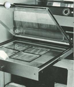
A photo printer produces patterns on circuit boards coated with photo-sensitive material.
