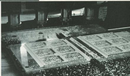
A numerically-controlled drilling machine automatically drills precise holes in printed circuit boards.
