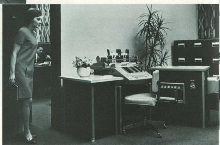
Thousands of California businesses of every size are users of Burroughs electronic and electro-mechanical accounting machines and systems. Systems such as the E 3500, above, feature electronic memories and computation, automatic data accumulation and report preparation.
