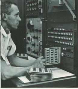
Quality control is assured by modern inspection equipment which automatically tests thirdgeneration, monolithic circuit boards.
