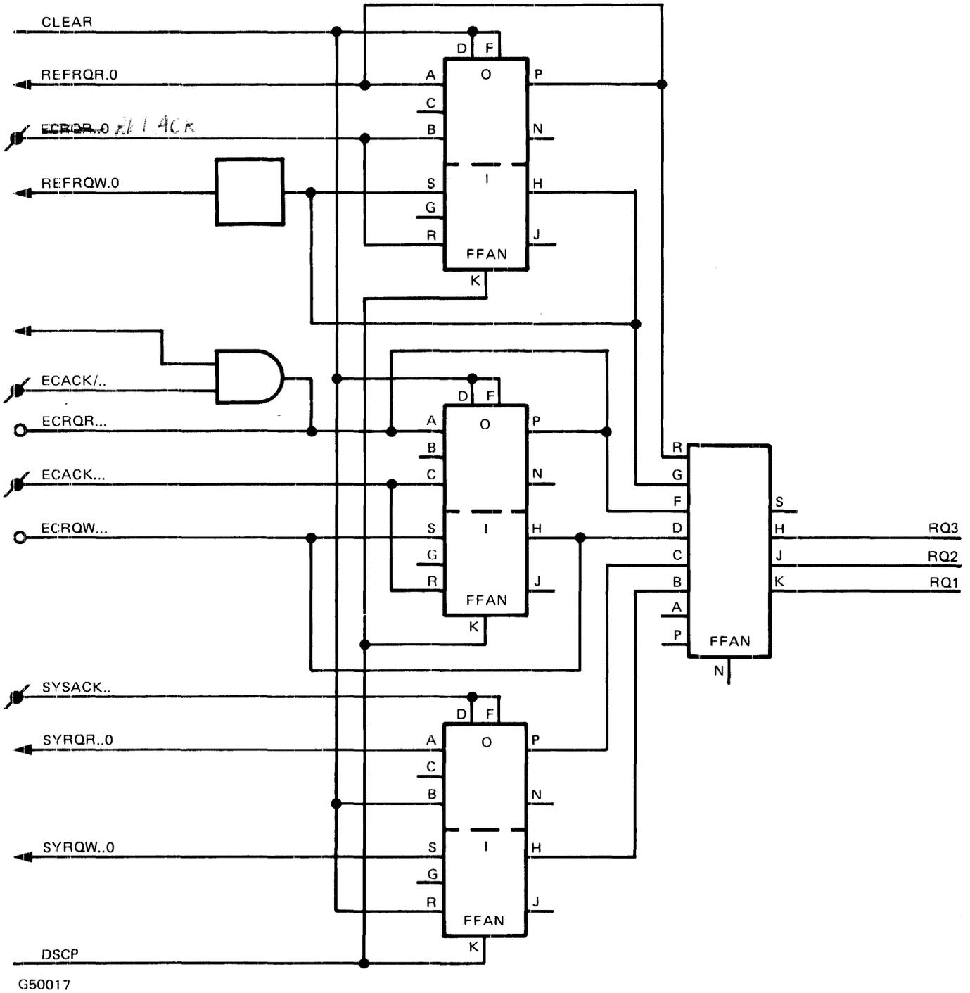
Figure 5-8. Memory Request Flip-flops and Priority Encoder
