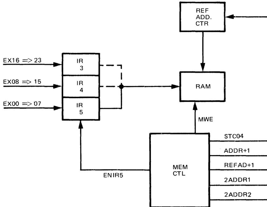
Figure 5-10. Reference Address Write Data Flow Diagram
