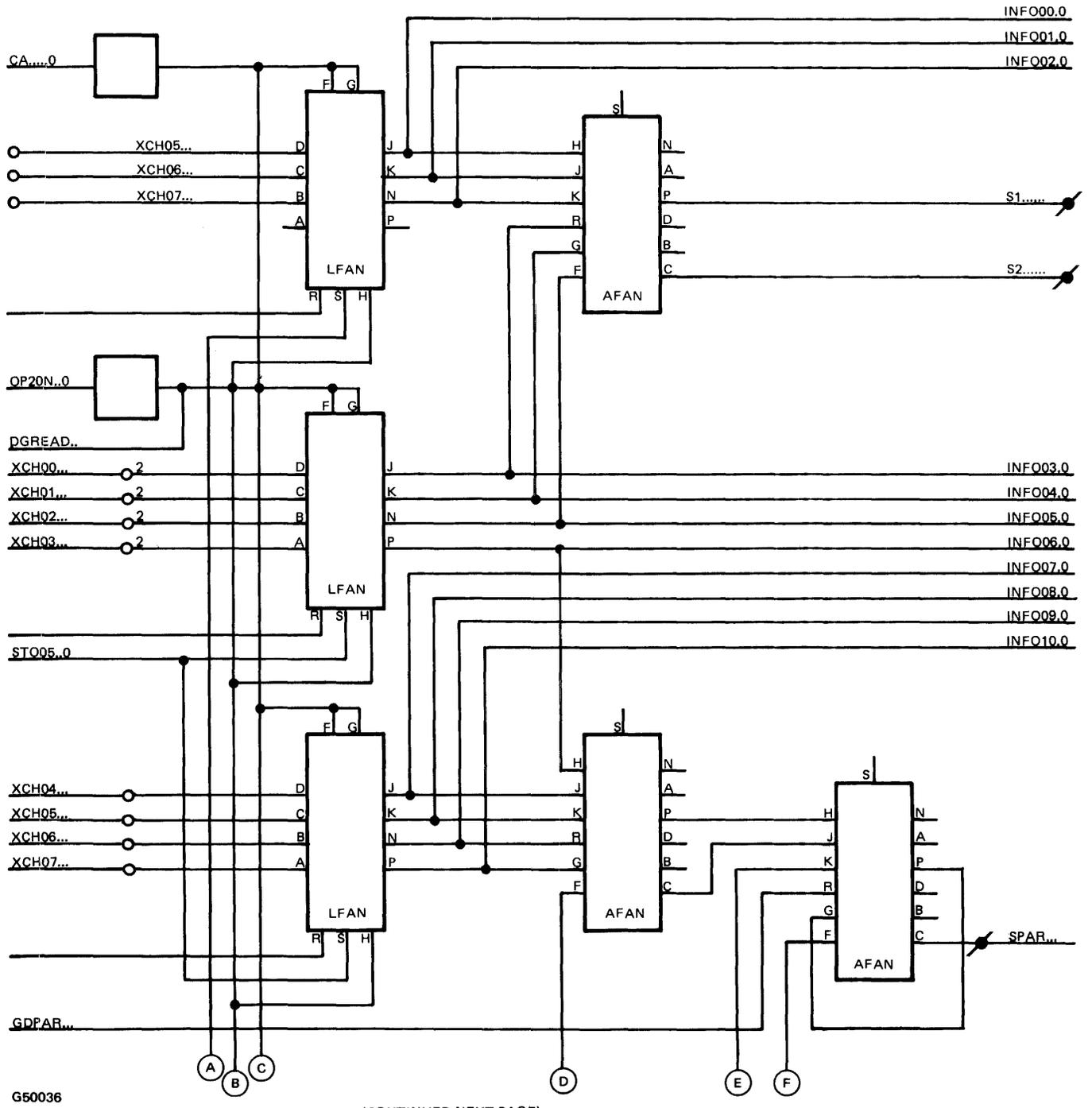
Figure 5-27. Parity Logic and File Address Register (Sheet 1 of 2)
