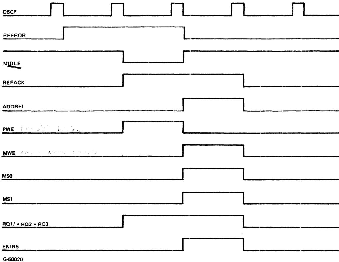
Figure 5-11. RAM Reference Address Write
