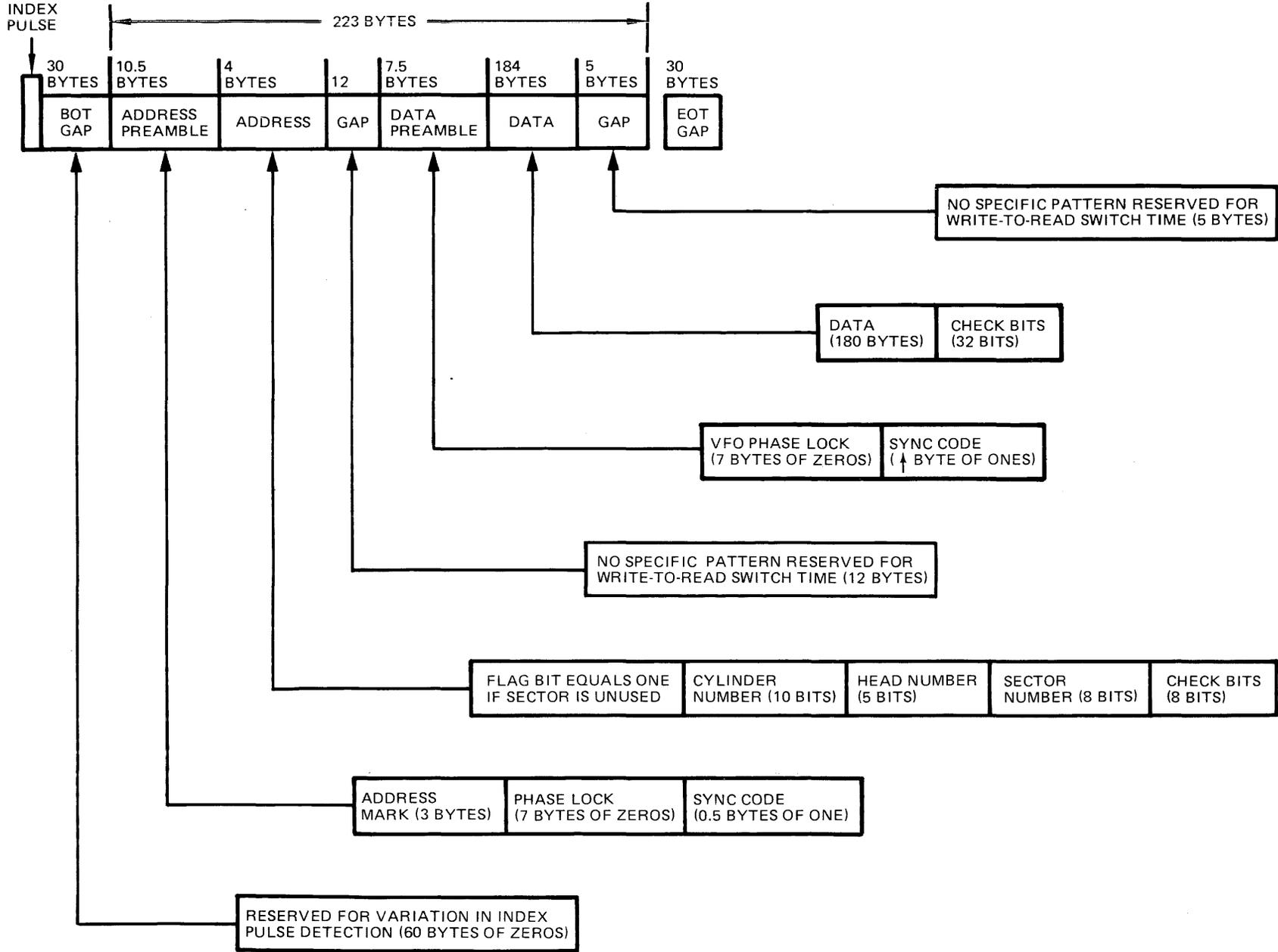
Figure 1-4. Type 206 Disk Pack Track Format
