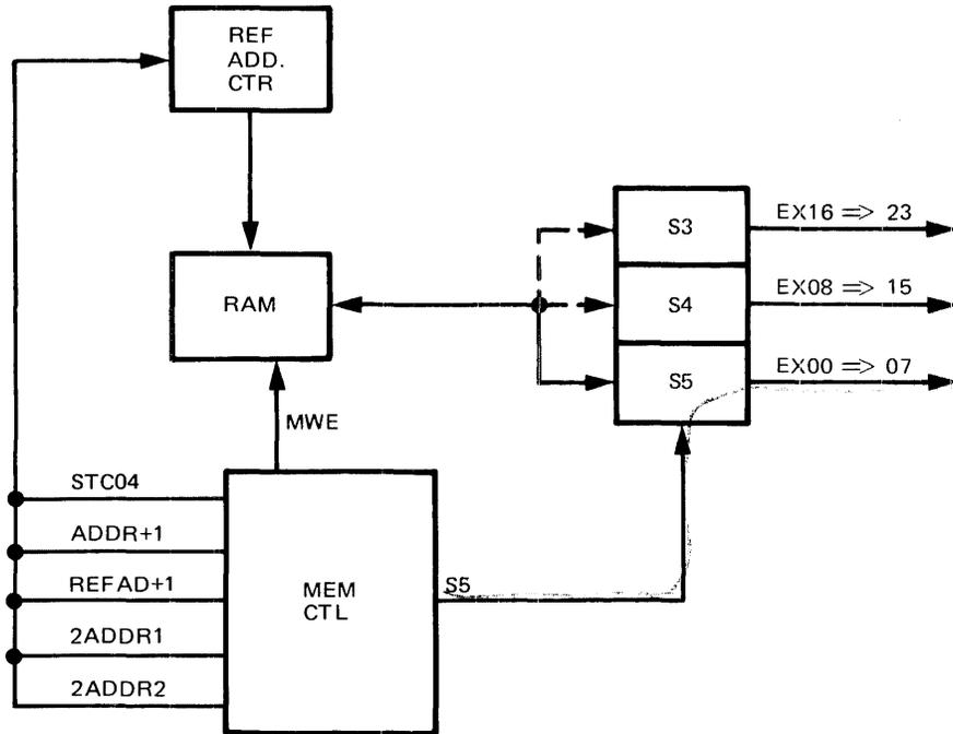
Figure 5-12. Reference Address Read Data Flow Diagram
