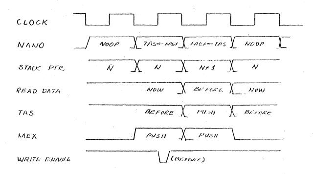
FIGURE 25 TIMING OF A-STACK OPERATION
