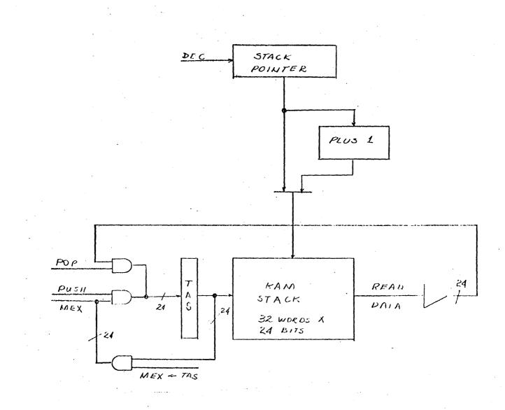
FIGURE 23 BLOCK DIAGRAM OF A-STACK
